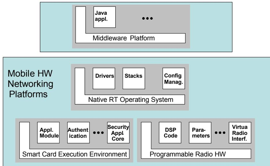
Fig. 2. Mobile Terminal Architecture
