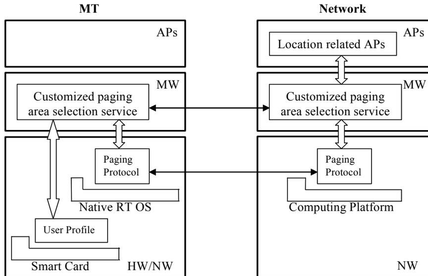
**Fig. 5.** Reference Architecture for Customized Paging Area
